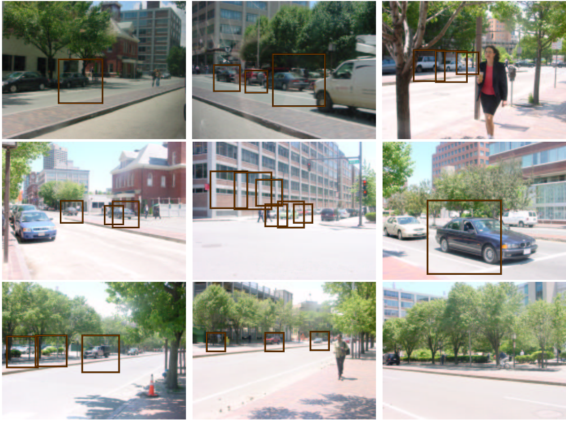
Figure 3-6: A detection task involving the StreetScenes shape-based objects. The C_1 features are used along with windowing and local neighborhood suppression in order to detect cars in full images. The system is charged with a false detection whenever the bounding box overlaps a unique ground-truth box by less than 50% of the union area. Several false-detections and false-negatives are visible in these images. Still, this task is very difficult, as there is no motion, and the cars may be at any pose without a pose-segmented training database. Note that the orange annotation squares are difficult to see without a color display.
