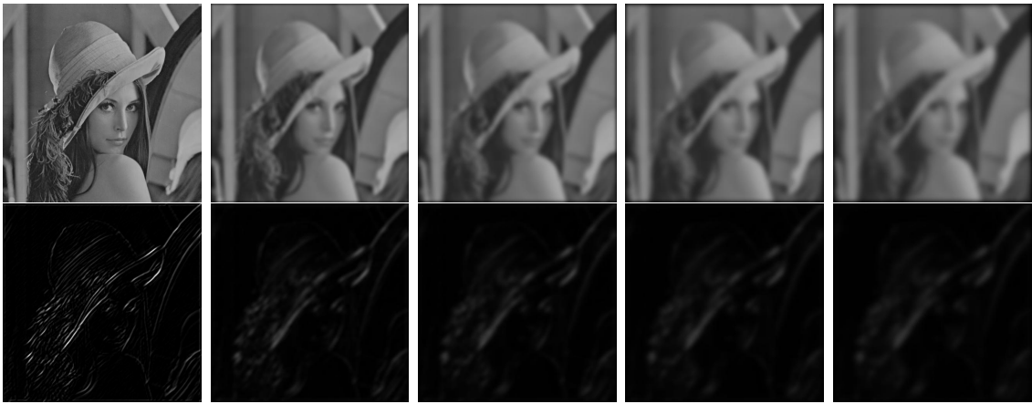
Figure 3-3: Gaussian scale-space images of Lena (top row) and of the gabor filtered version of Lena (bottom row). While the gray-value image degrades gracefully, revealing structures at different scales, the sparse edge image fades away.
